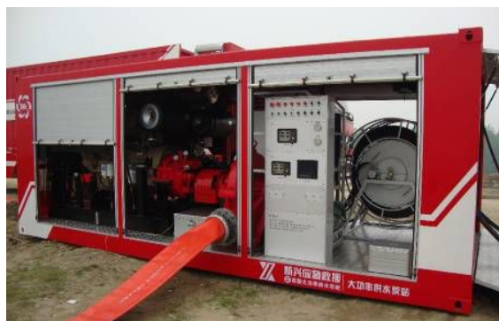
Figure 2: Pumping station shelter
