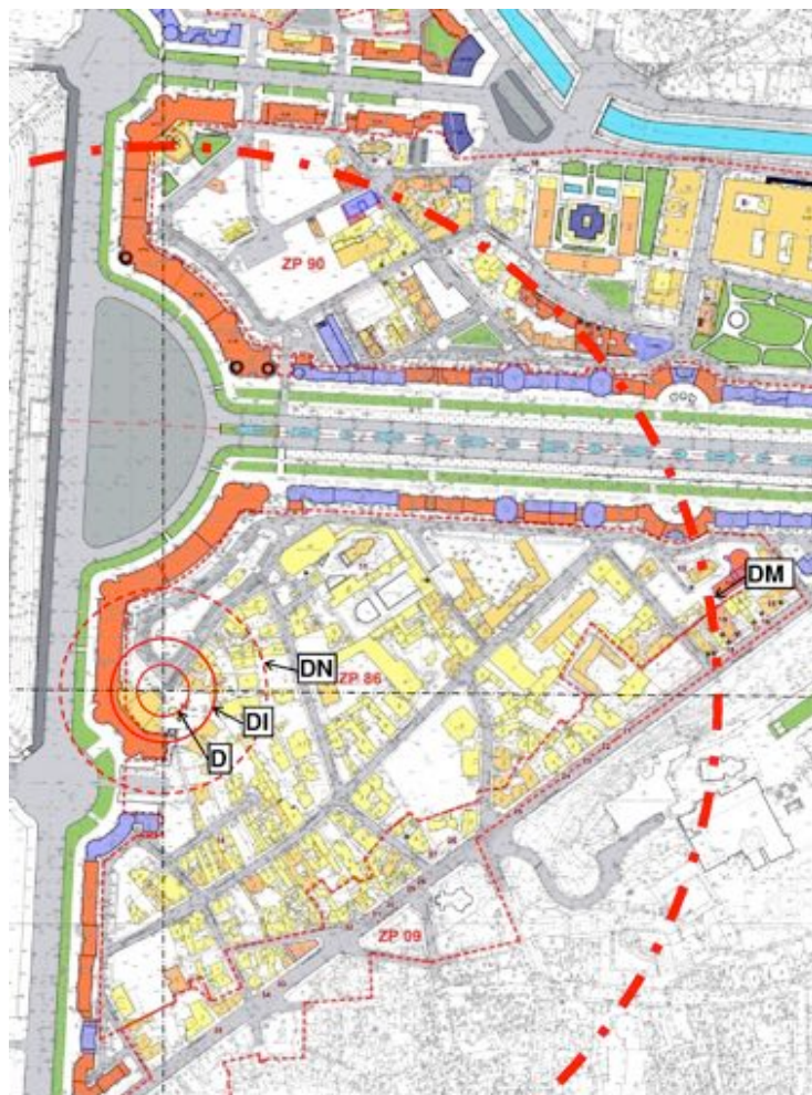
Figure 9 Radiuses of specific zones in a specific location within the study area. Position B – Scenario S 4.4 - case 3 –explosive in quantity to be carried by a urban van.
