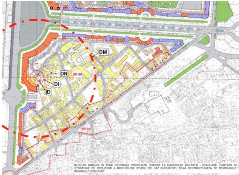
Figure 8 Radiuses of specific zones in a specific location within the study area. Position B – Scenario S 4.4 - case 2 –Explosive in quantity to be carried by a compact car.
