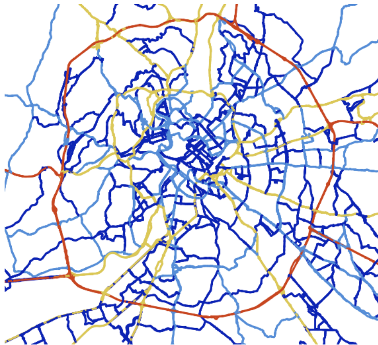
Figure 1: Tele Atlas MultiNet graph up to Net2Class=3 in the city of Rome. Color scale varies from blue to red according to the Net2Class index. Red streets are more important than blue ones as they exhibit lower Net2Class score. The urban street network of Rome is built on a metropolitan freeway that surround the city, (Grande Raccordo Anulare or GRA) which correspond to the big red circle in the figure, and some other fast streets connecting GRA to the city center.
