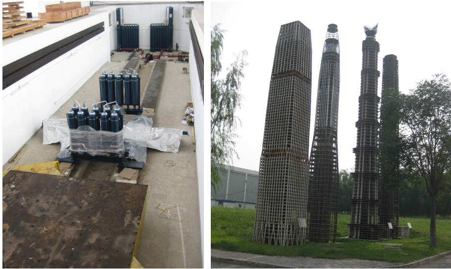
Figure 6 The shaking table in construction at IEM-Yanjiao (left); Models of super-high buildings recently made, scale 1:40, after testing at China Academy of Building Research, Platform Yanjiao (right)
