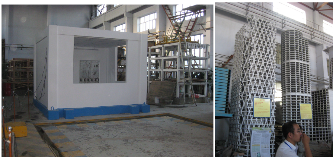
Figure 8 Institute of Engineering Mechanics - IEM Harbin, China. Models prepared for 3 D seismic tests on
