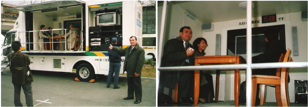
Figure 11 Mobile seismic simulator during WDRR, Kobe, Japan, 2005 (left). Persons on the platform are subjected to a seismic motion in successive steps. Seated position gives greater stability, so it can reach up to 6 degrees of intensity JMA Japanese Scale (2.5 ... 3.15 m/s 2 ; 3.15 ... 4.00 m/s 2 ; for indicative comparison, Vrancea earthquake recording March 4th, 1977 at INCERC reached to 2.07 m/s 2 ), Japan
