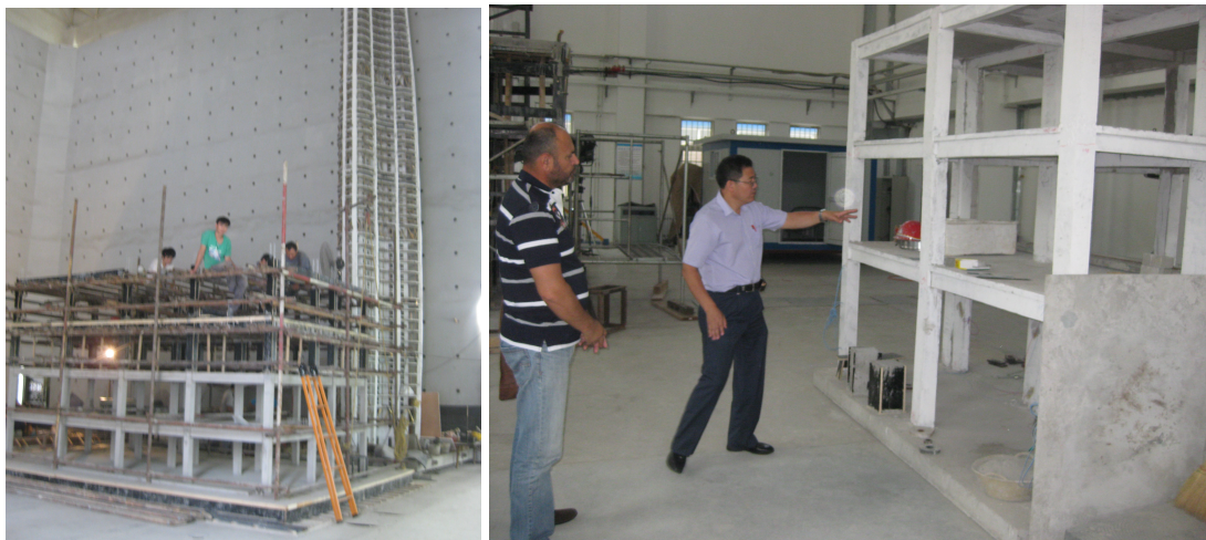
Figure 7 Models of buildings in preparation for testing on shaking table/seismic simulator at China Academy of Building Research (left); model of structure prepared for testing on shaking table(right)
