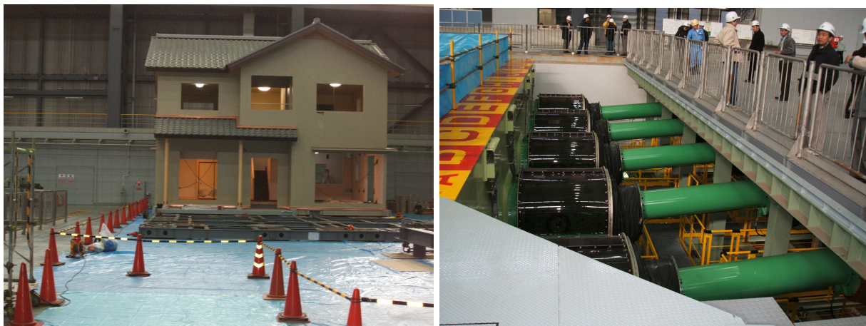
Figure 5 E-Defense NIED Shaking Platform, Miki Town, Japan; the actuators
