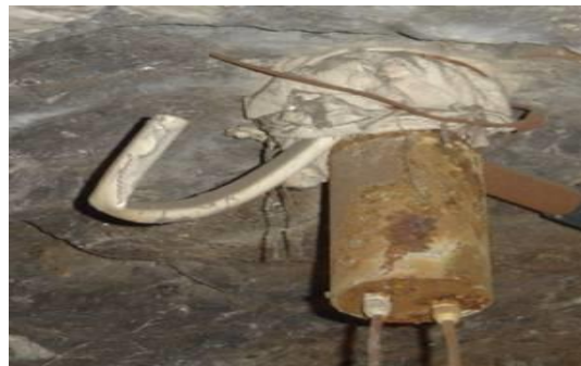
Figure 10. Field test scene of multiple point displacement meter
