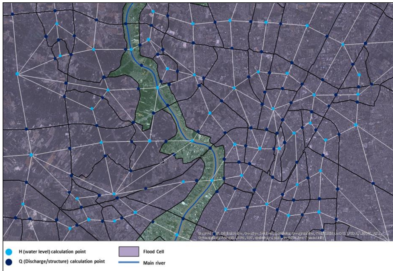
Figure 3 Quasi-2D schematization proposed for the floodplain
