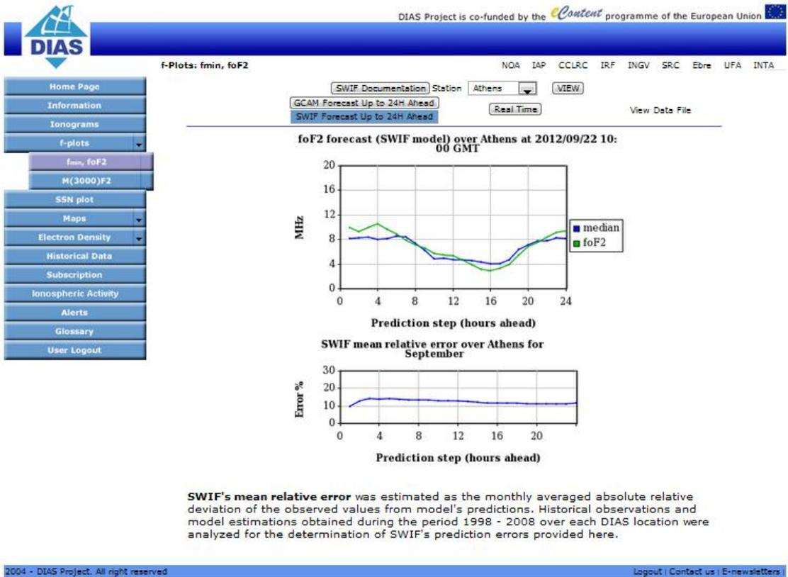
Figure 5: In the screenshot above we present an indicative example of the foF2 forecasts for the next 24 hours over Athens based on the SWIF model with the mean relative error for each prediction step.
