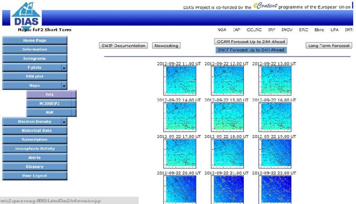
Figure 2: A screen shot from the DIAS portal, showing the calculated maps of foF2 forecasts for the next 24 hours. Predictions are calculated with the SWIF model (Solar Wind Driven Ionospheric Forecast) and for the mapping the SIRMUP model is applied. SWIF forecasts are updated hourly.
