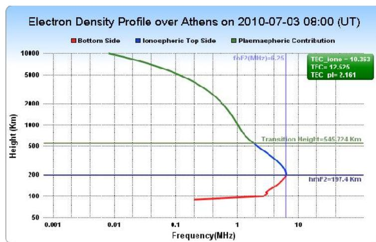
Figure 6: An example of reconstructed electron density profile over Athens Digisonde applying the TaD model. Red line corresponds to Digisonde bottomside reconstructed profile. The topside is extrapolated with TaD algorithm. The blue part corresponds to the topside and the green part to the plasmasphere. It is possible with this analytical approach to calculate partial TEC that corresponds to the topside and to the plasmaspheric part.
