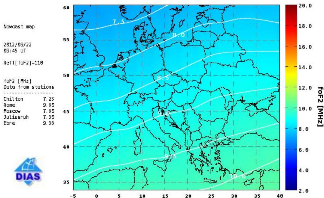
Figure 1: An example of a regional foF2 nowcasting map on 22/9/2012 at 09:45 UT which has been generated using the ionospheric data from the DIAS sounders, based on the SIRMUP model. The estimated value of the effective sunspot number as well as the real-time values of the foF2 parameter observed from the DIAS stations are given on the left hand side.
