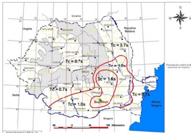
Figure 10. Zonation of the Romanian territory in terms of control period (corner period) T_C of the response spectrum
