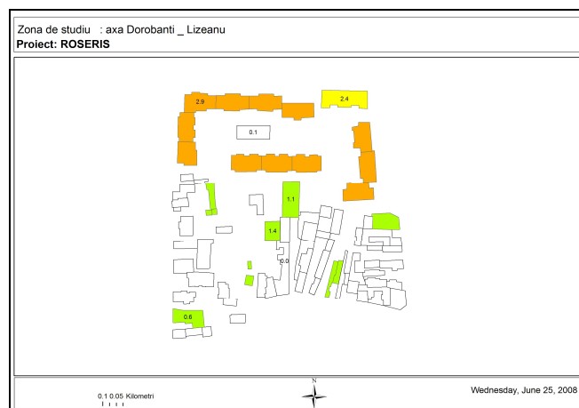
Figure 6. Mean damage ratios, GMA, for the buildings in the pilot zone
