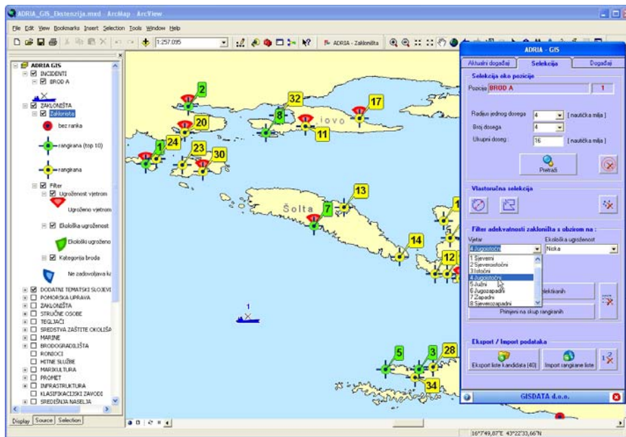
Figure 6: GIS + additional extension: Elimination (red triangle) of those PoR that have low protection from south-east wind
