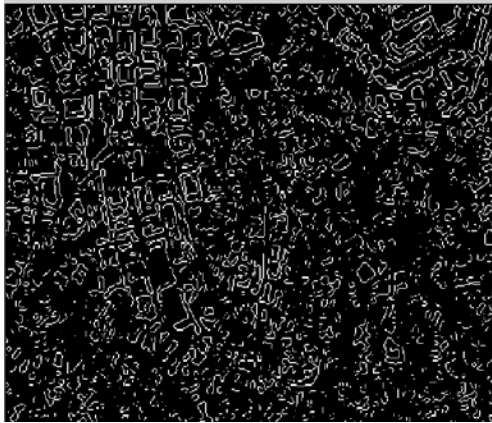
Edges defined with Zero-Cross Algorithm
