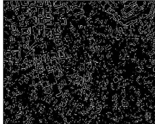
Edges defined with Laplacian of Gaussian Algorithm
