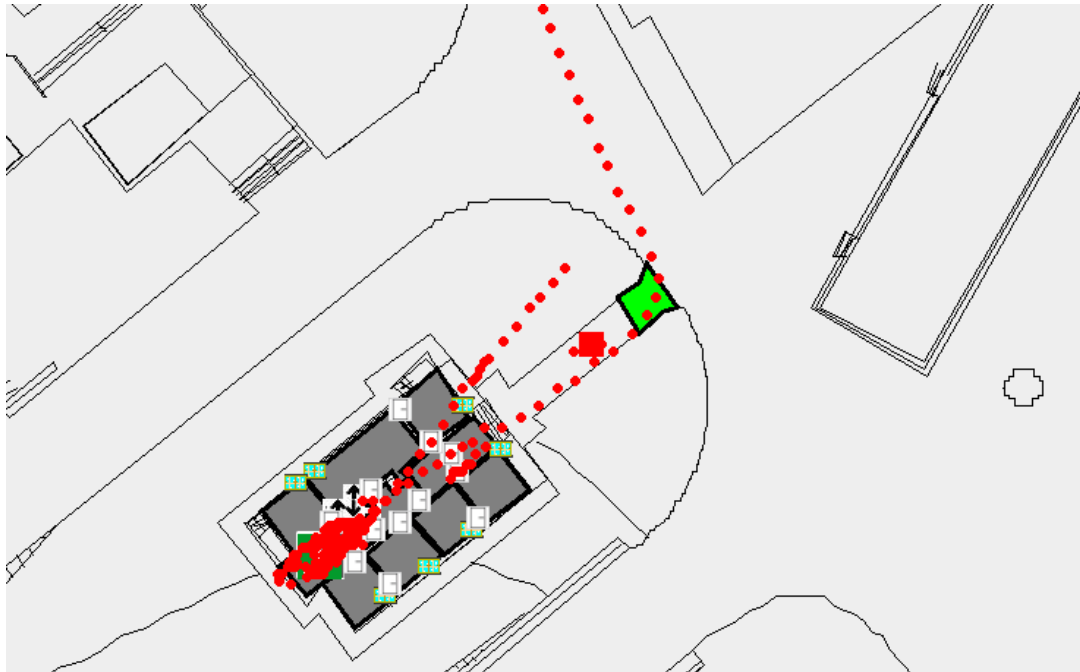
Figure 3: MEMS, and AGPS location based technique with calibration inside the Fire House
