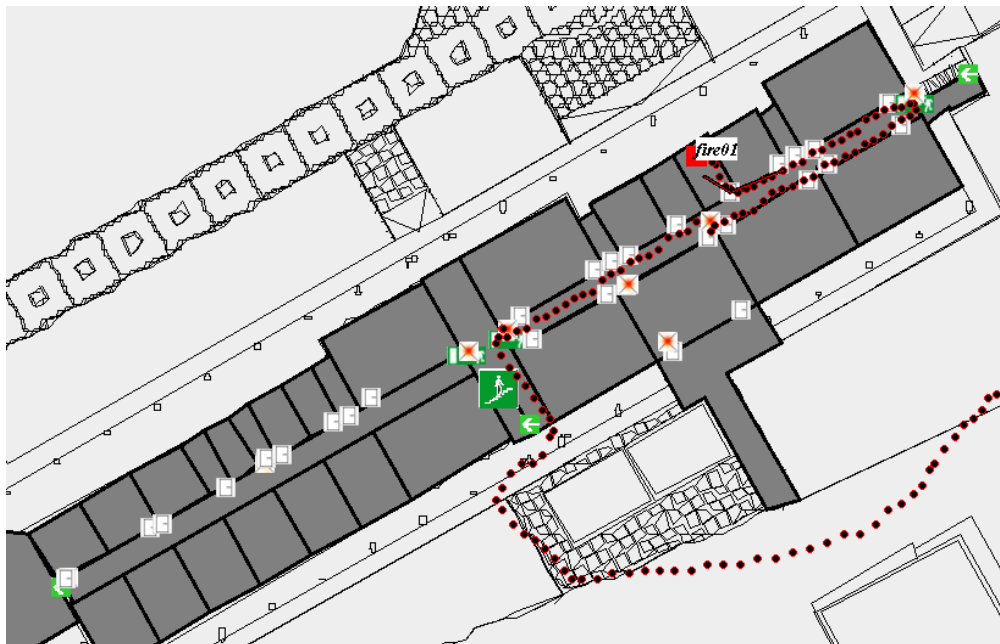
Figure 2: MEMS, and AGPS location based technique with calibration inside the Main Building
