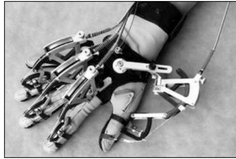
Figure 3: Example of tactile device for telesurgery
