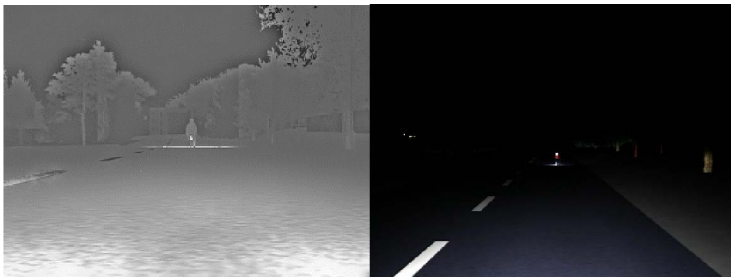
Figure 7: Night, clear weather. Cyclist is completely visible with SEE, but only a back-light is visible without SEE, i.e. missing back light means no sight of the cyclist without the SEE system.
