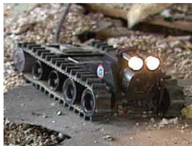
Figure 1: Example of search and rescue robot (NSF PR 03-91, downloaded from http://www.nsf.gov/od/lpa/news/03/pr0391.htm )
