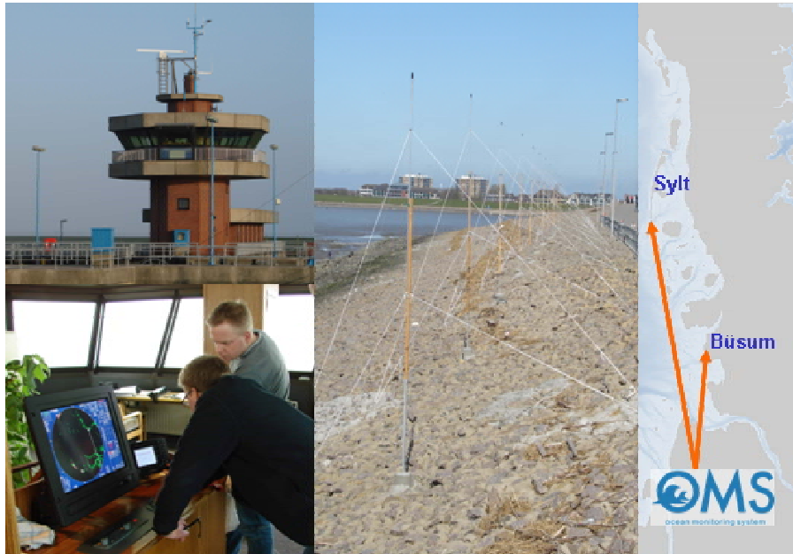
Figure 3: Locations and illustrations of the X-Band and HF-SWR Radar systems of the OMS. The two photos on the left show the site of the X-Band and wave monitoring radar installation at the port lock building of Büsum. The photo on the right shows the HF-SWR radar antennas installed in Büsum. Photos courtesy of Raytheon Anschütz GmbH and Helzel Messtechnik GmbH.
