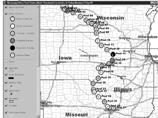
Figure 6. ENGLink-delivered map showing daily status of levees on the Mississippi River during spring flood.
