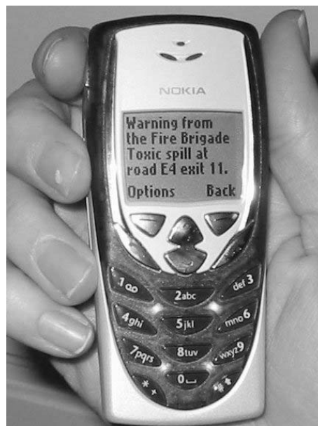
Figure 2: Example of a warning message sent using Short Message Service (SMS) and received on a cellular phone.
