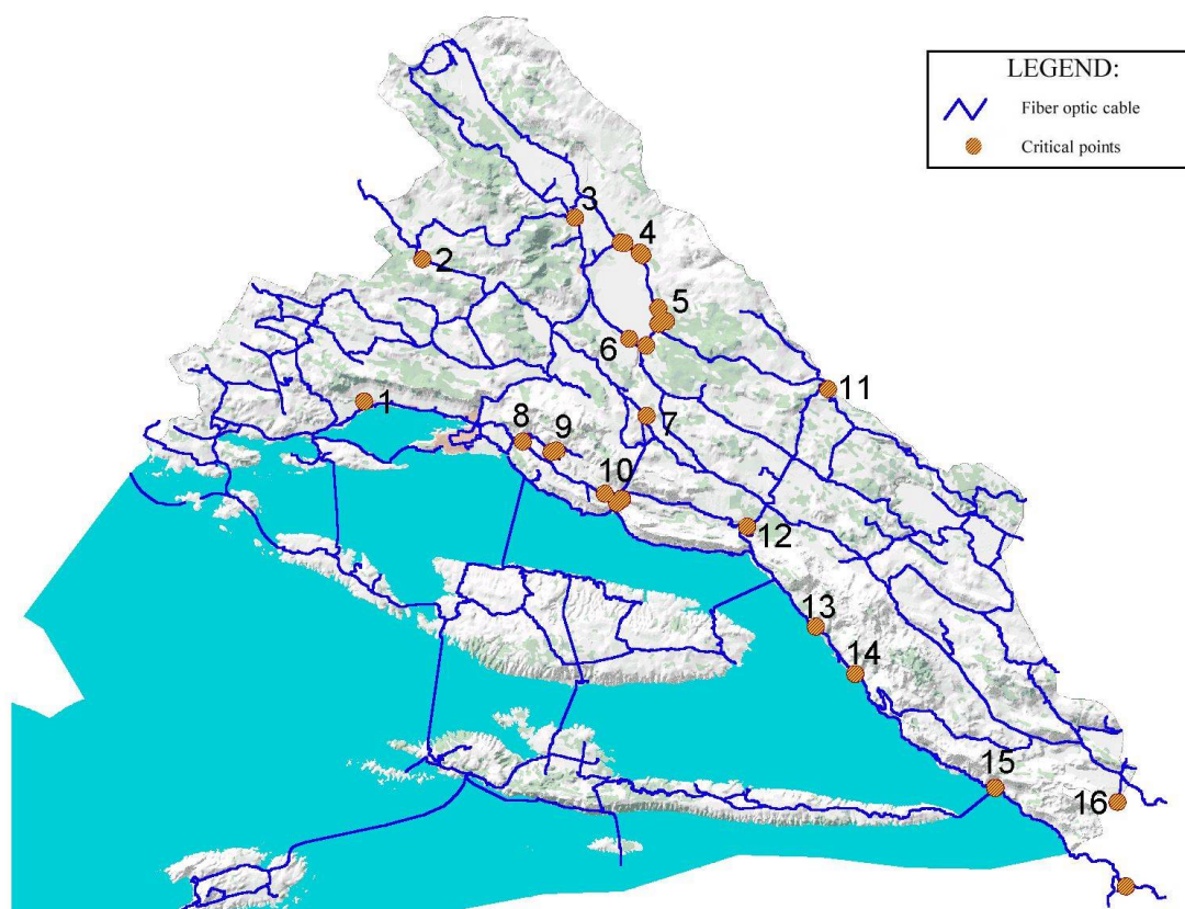
Figure 4. 3D layout of County and critical points with regard to the danger from lightning (besides high-voltage networks) and torrents
