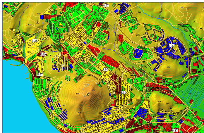
Fig. 2. Damage extent due to scenario event for Petropavlovsk-Kamchatsky City (black color -total collapse, brown - partial collapse, red - heavy damage, yellow -moderate damage, green - slight damage, blue - no damage)
