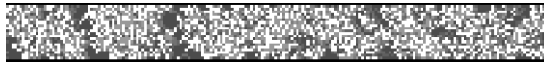
Figure 6: Corridor with periodic boundary conditions and a density of 4,4 \text{ P/m}^2 . People are moving from the left to the right and occupying only one cell. Jam-waves are clearly visible (dark areas).
