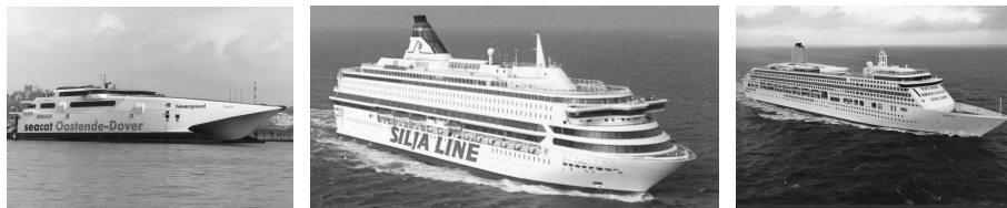
Figure 1: Pictures of a typical HSC, a RoPax-Ferry and a cruiseliner (pictures: author, Jos. L. Meyer shipyard).
